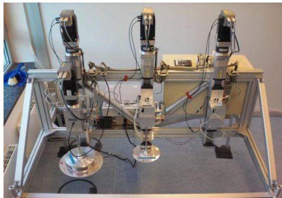
Fig. 3. Bevameter with loading plates of various size (applied force of 500 N) [14]
