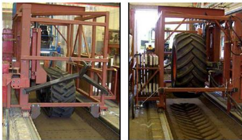
Fig. 8. Laboratory soil bin. Rubber track (left) and harvester tire (right) [1, 5]
